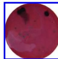
Figure 13. CuO disk after the reaction by catalyst disk with 96 Ni spots.
