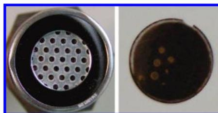
**Figure 9.** Pt/Al<sub>2</sub>O<sub>3</sub> in punched holes of aluminum plate and detector disk after reaction.
